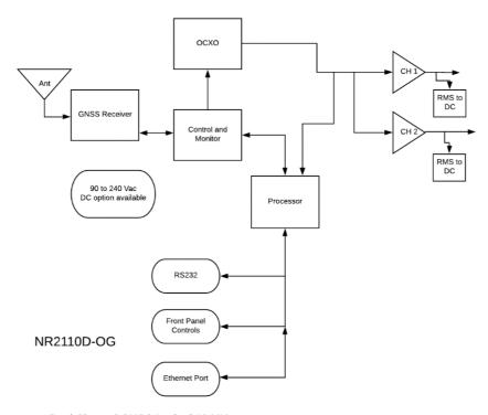
Dual Channel GNSS Locked 10 MHz Rubidium Reference
