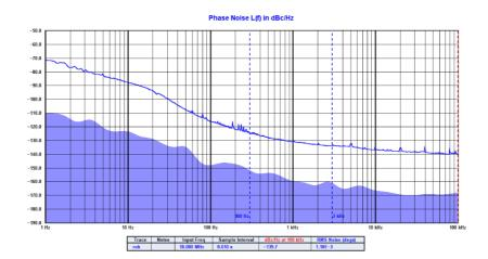
For applications requiring the stability of an atomic source but also requiring low phase noise, a low phase noise OCXO is disciplined to an atomic source. The phase noise for the NR2110-R/O has phase noise improved by well over 20 dB by this technique.
