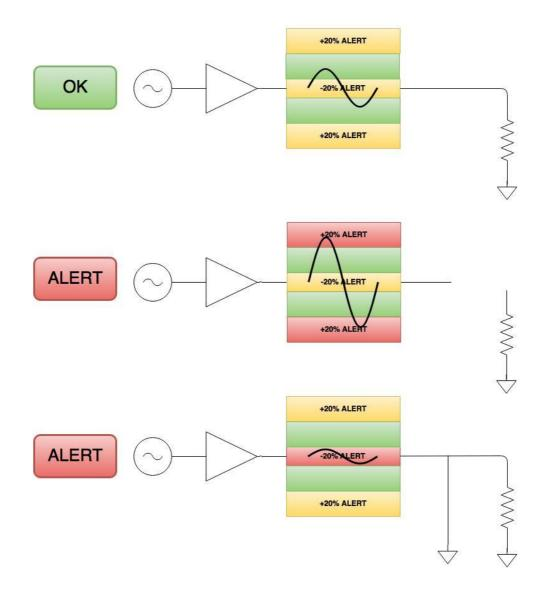
The Alert Threshold can be optimized so that a channel short or an impedance change will cause an Alert.
