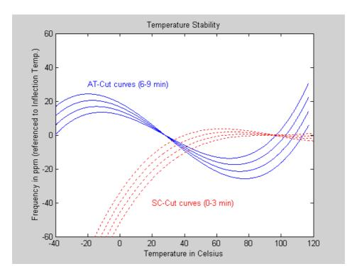
Over a broad temperature range, an AT performs very well and much easier to compensate electronically. It is also a simpler crystal to manufacture than a SC cut device. For applications where a stability of a few ppm is acceptable, a TCXO can be a cost-effective alternative.
