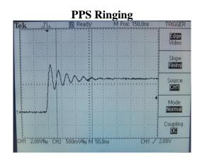
If properly terminated – a 50 Ohm cable can be used, but most CMOS drivers will not drive a 50 Ohm load. If the load is 5 Vdc CMOS at 50 Ohms, then the drive current is approaching 100 mA. This high drive current also compounds the short circuit protection that is essential in any complex system. Short run, high impedance cabling can work if done so carefully. Other options include LVDS. LVDS works very well < 20 meters and is offered on several references.
