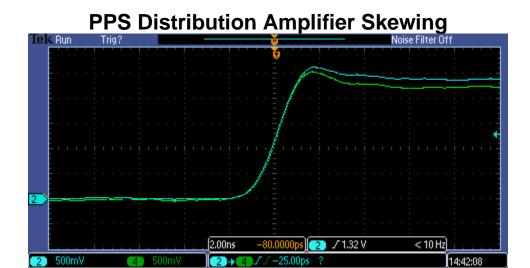
Fiber optic distribution systems are available for PPS, but edge dispersion can compromise accuracy. Single mode systems must be considered but are more costly. Depending upon the receiver used, the relationship between the PPS rising edge and the NMEA data varies. The rising edge may be for the NMEA data stream received or for the NMEA data that will be received next.
