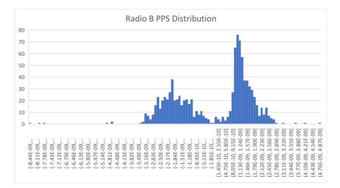
Depending upon the locking algorithm, the radio PPS variation can contribute directly to phase noise and instability.
