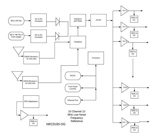
There is built-in test circuitry throughout the design. Power supplies, signal present are monitored and are used to drive a status relay as well as indicators on the front panel and optional serial and Internet communications paths.
