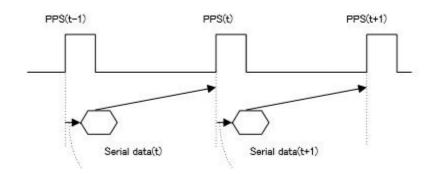
The serial data timing is for the next rising edge of the PPS pulse.
