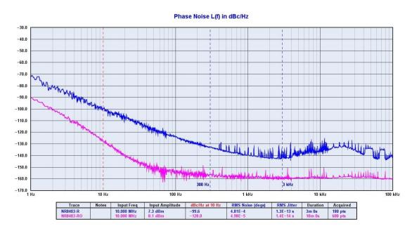
Our Rubidium references offer a stability of < ±1 ppb/year compared to a typical OCXO ±50 ppb/year. The Rubidium source consists of a voltagecontrolled crystal oscillator (VCXO) which is locked to a highly stable atomic transition in the ground state of the 85Rb isotope.
