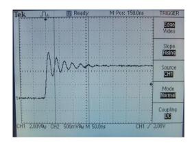
If properly terminated – a 50 Ohm cable can be used, but most CMOS drivers will not drive a 50 Ohm load. If the load is 5 Vdc CMOS at 50 Ohms, then the drive current is approaching 100 mA. This high drive current also compounds the short circuit protection that is essential in any complex system. Short run, high impedance cabling can work if done so carefully. Other options include LVDS. LVDS works very well < 20 meters and is offered on several references.
