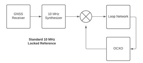
The standard loop does an outstanding job of controlling an OCXO. Components such as GaAs mixers provide excellent phase measurement performance, but close-in phase noise is difficult due to the size of the filtering components required and attendant leakage currents which are limited by the mixer drive currents.
