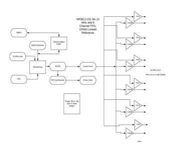
The NR3612-O/G is a high performance 10 MHz GNSS locked, OCXO based frequency reference that features 6 channels of 10 MHz and 6 channels PPS
