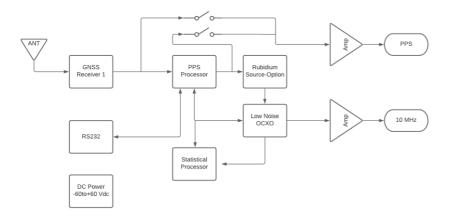
Single Channel GNSS locked reference featuring high stability. The unit also features a PPS source with a standard deviation of under 5 ns. Pulse to pulse jitter is well under 200ps. In addition to output amplitudes and internal critical measurements, the unit reports a continuous calculation of Allan Deviation. Various phase noise options are available. requirements. Operates from -60 to +60 Vdc in three ranges.
