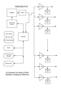
Stable Rubidium source provides 10 channels of 10 MHz sine or (optionally) ten MHz square. All channels are monitored for a fault or open condition. Low noise OCXO locked to the Rubidium dominates phase noise performance.
