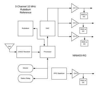
This reference brings exceptional stability in an economical package. There are three 10 MHz outputs plus a PPS and NMEA. External locking options allows the unit to be locked to an external PPS or 10 MHz reference. The unit is available as a 10 MHz reference or 50 MHz.
