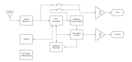
Single Channel GNSS locked reference featuring high stability. The unit also features a PPS source with a standard deviation of under 5 ns.. In addition to output amplitudes and internal critical measurements, the unit reports a continuous calculation of Allan Deviation. Various phase noise options are available. requirements. Operates from -60 to +60 Vdc in three ranges. Pulse to Pulse jitter < 1 ns
