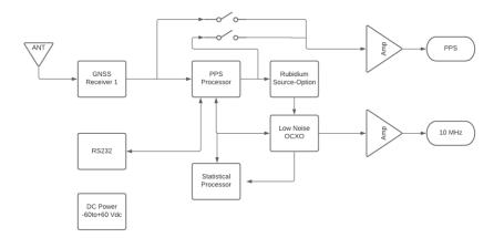
Single Channel GNSS locked reference featuring high stability. The unit also features a PPS source with a standard deviation of under 5 ns. In addition to output amplitudes and internal critical measurements, the unit reports a continuous calculation of Allan Deviation. Various phase noise options are available. requirements. Operates from -60 to +60 Vdc in three ranges.
