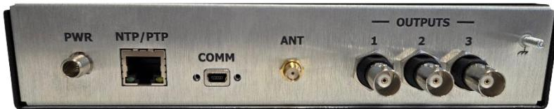
GNSS Locked PTP Time server provides nanosecond time for the entire network. User selectable 3 channel timing outputs with options for 10MHz, PPS, or IRIG signals.
