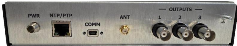
GNSS Locked NTP Time server provides usec time for the entire network.
